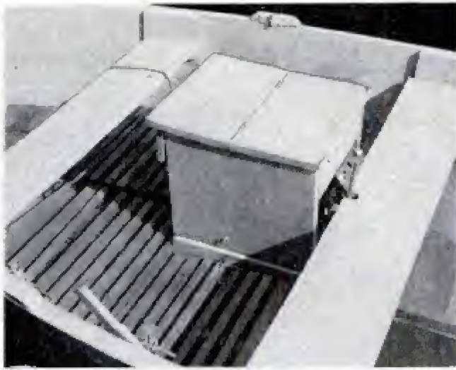
Top of the engine cover or hood should be hinged for easy access to starting cord. Note the open ends
